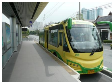
Figure 16.8-6: Precise docking with guidewheel system
